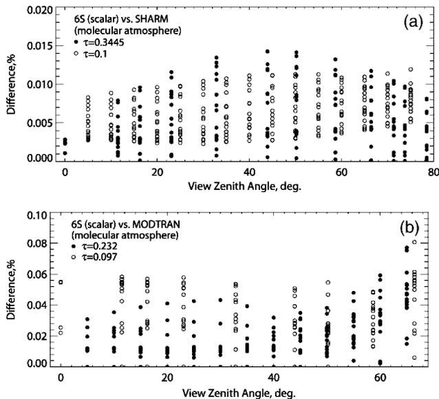
Fig. 2. Validation of 6SV1 in scalar mode against (a) SHARM and (b) MODTRAN for a molecular atmosphere. (a) SZA = {0.0°; 10.0°; 23.07°; 45.0°; 58.67°; 75.0°}, AZ = {0.0°; 90.0°; 180.0°}, VZA = {0°–79°}, optical thickness of  $\tau = \{0.1; 0.3445\}$ , surface reflectance of  $\rho = 0$ . (b) SZA and VZA sets do not include angles beyond 70°,  $\tau = \{0.097; 0.232\}$ ,  $\rho = 0$ .
