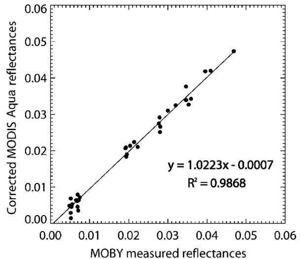
Fig. 9. Corrected MODIS Aqua water-leaving reflectances versus the MOBY-measured water-leaving reflectances for  $\lambda = \{412; 443; 490; 530; 550\}$  nm. MOBY data were collected off the coast of Lanai Island, Hawaii, during 2003.
