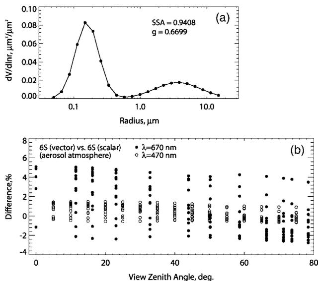
Fig. 7. (a) Average volume size distribution of particles for a biomass burning smoke aerosol model. (b) Effects of polarization for an aerosol atmosphere represented by the biomass burning smoke.  $SZA = \{0.0^\circ; 11.48^\circ; 23.07^\circ; 32.86^\circ; 58.67^\circ\}$ ,  $AZ = \{0^\circ; 90^\circ; 180^\circ\}$ ,  $VZA = \{0^\circ-79^\circ\}$ ,  $\tau = 0.728$  (hazy conditions),  $\lambda = \{470; 670\} \text{ nm}$ .
