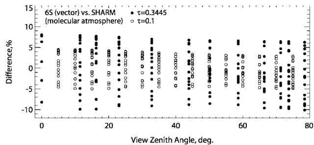
Fig. 6. Effects of polarization for a molecular atmosphere.  $SZA = \{0.0^\circ; 10.0^\circ; 23.07^\circ; 45.0^\circ; 58.67^\circ; 75.0^\circ\}$ ,  $AZ = \{0.0^\circ; 90.0^\circ; 180.0^\circ\}$ ,  $VZA = \{0^\circ-79^\circ\}$ ,  $\tau = \{0.1; 0.3445\}$ ,  $\rho = 0$ .
