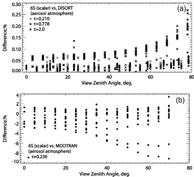
Fig. 3. Validation of 6SV1 in scalar mode against (a) DISORT and (b) MODTRAN for an aerosol atmosphere. (a) Standard continental aerosol model. SZA = {0.0°; 10.0°; 23.07°; 45.0°; 58.67°; 75.0°}, AZ = {0.0°; 90.0°; 180.0°}, VZA = {0°–79°}, optical thickness of  $\tau = \{0.210; 0.778; 2.0\}$ , surface reflectance of  $\rho = 0$ . (b) Clean continental aerosol model. SZA and VZA sets do not include values beyond 70°,  $\tau = 0.236$ ,  $\rho = 0$ .
